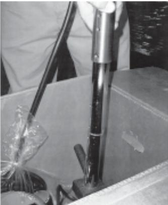
4. Lift upper handle and place end-to-end against lower handle, lining up the holes for the bolts. Slide handle sleeve downward until all holes are lined up.
