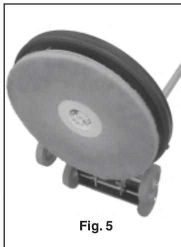
**CAUTION:** Disconnect the power cord from the electrical outlet before installing a brush or pad driver.
