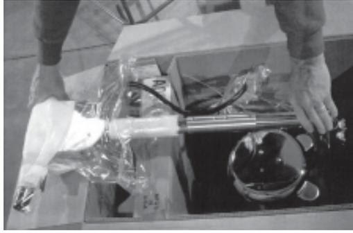
2. Move upper handle forward to expose wing nuts and angle bracket.
