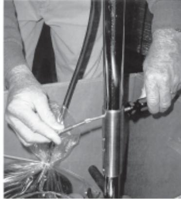
5. Use a screwdriver to line up holes and guide bolts through the handle.
