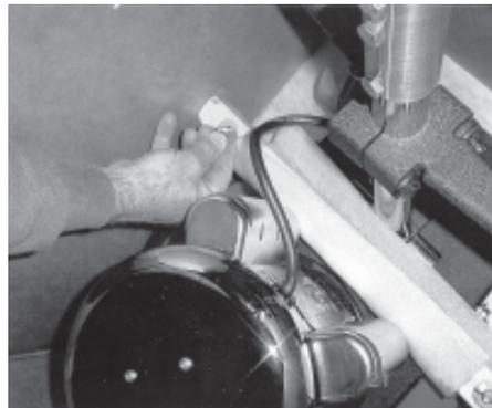
8. Remove wing nuts and washers to unfasten wood shipping retainer. Discard wood shipping retainer.
