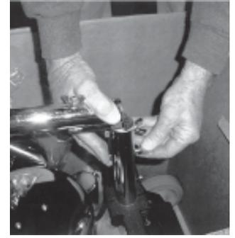
3. Remove the wing nuts and bolts from both upper and lower handle. Discard the angle bracket.
